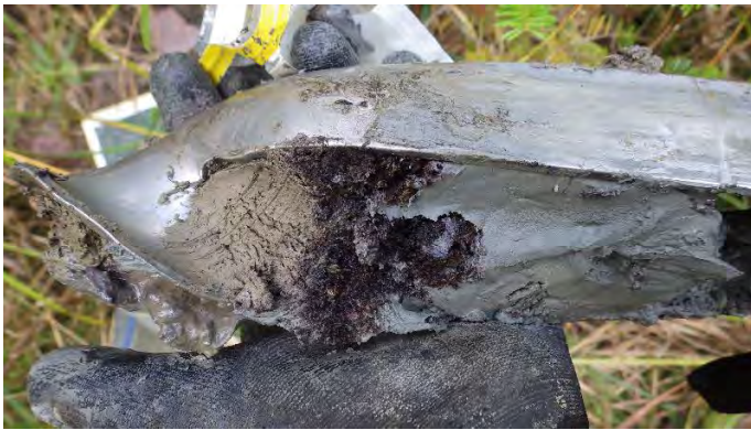
Figure 3.55: A soil core revealing soils buried by a landslide in Lyman, Maine. The darkest layer in the middle of the core was the topsoil and the grey layer on the right was the bottom of the landslide (in this case, consisting of Presumpscot Formation). Plant fragments from the buried soil layer were sent for radiocarbon analysis to estimate the landslide age. Photo: Maine Geological Survey.
