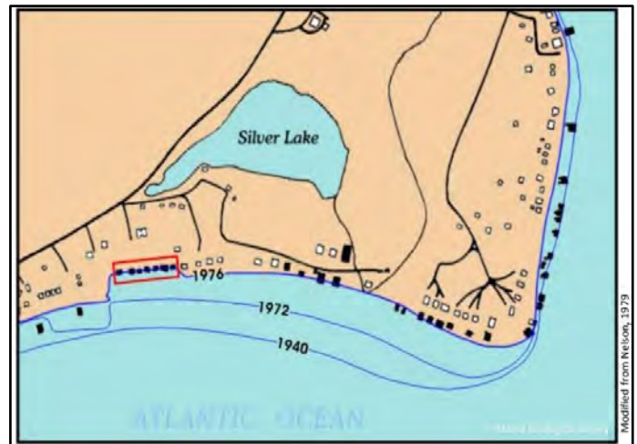
Figure 3.44: Historic shorelines along Popham Beach in Phippsburg. The blue lines show the location of the shoreline in 1940, 1973, and 1976. The small rectangles represent houses along the coast. The black rectangles represent houses that have been destroyed due to the coastal erosion. The red box outlines a row of
